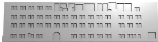
(b) 3D façade model after data-driven reconstruction
